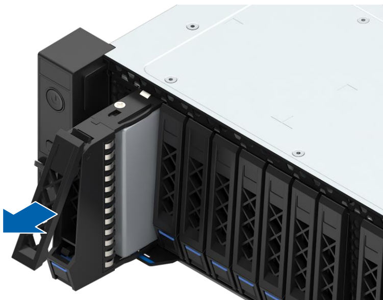
Figure 4-32 Pulling out the Drive Module
