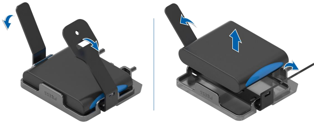
Figure 4-4 Removing the Super-Capacitor
