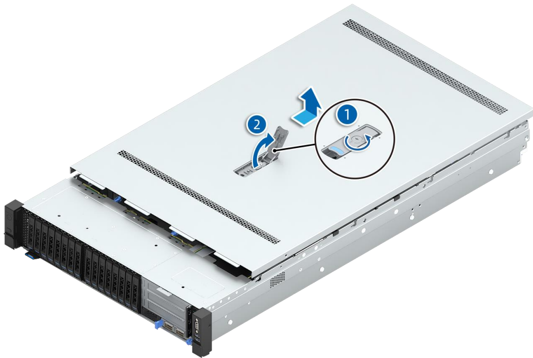
Figure 4-3 Removing the Top Cover
