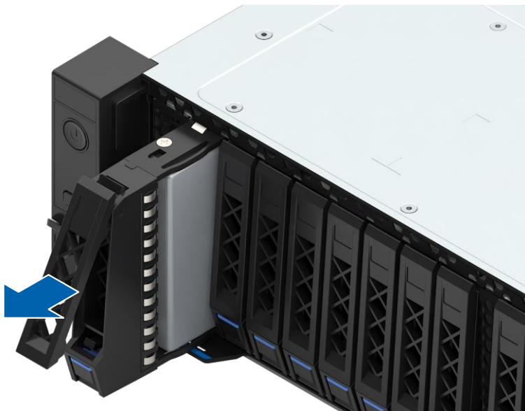
Figure 4-32 Pulling out the Drive Module
