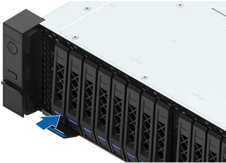
Figure 4-31 Pressing the Release Button
