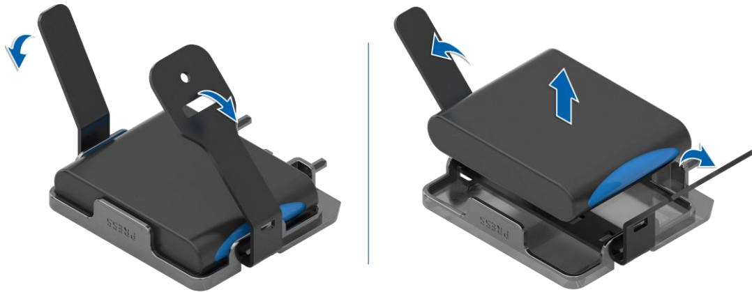
Figure 4-4 Removing the Super-Capacitor
