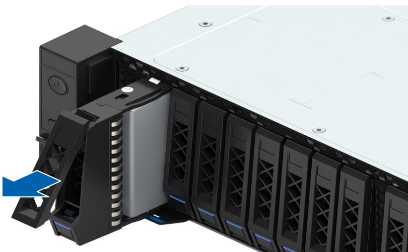
Figure 4-32 Pulling out the Drive Module
