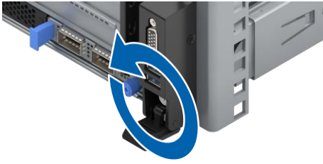
Figure 4-1 Loosening the Captive Screw
