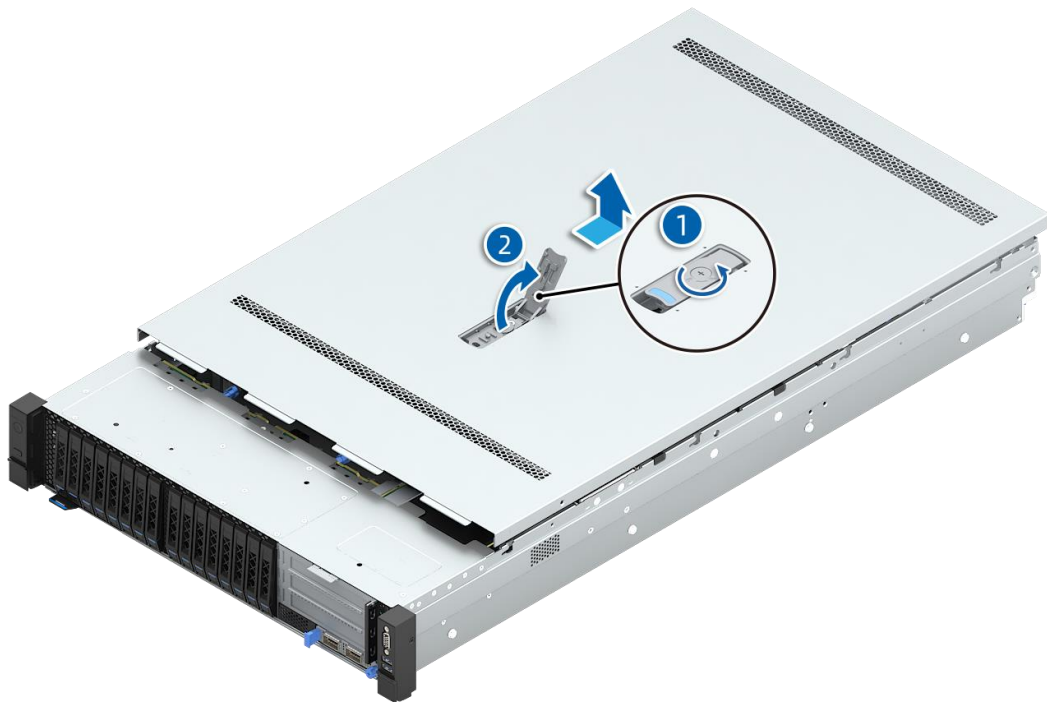
Figure 4-3 Removing the Top Cover
