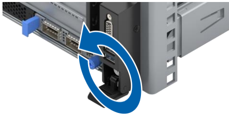
Figure 4-1 Loosening the Captive Screw
