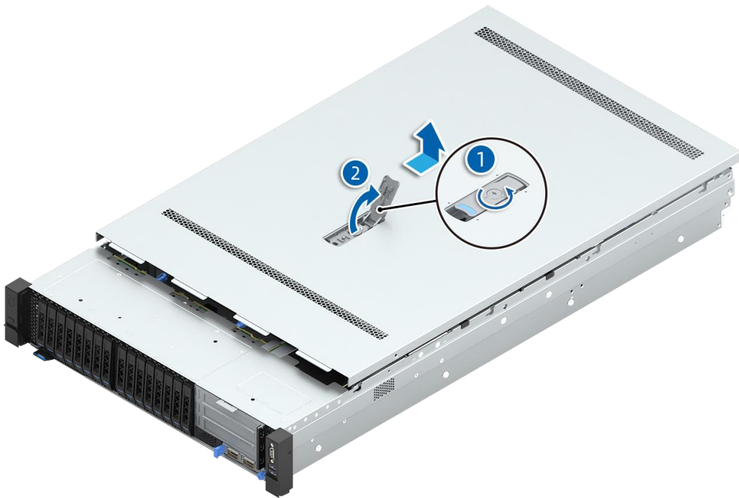
Figure 4-3 Removing the Top Cover
