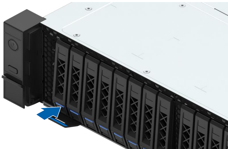
Figure 4-31 Pressing the Release Button
