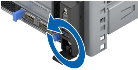
Figure 4-1 Loosening the Captive Screw
